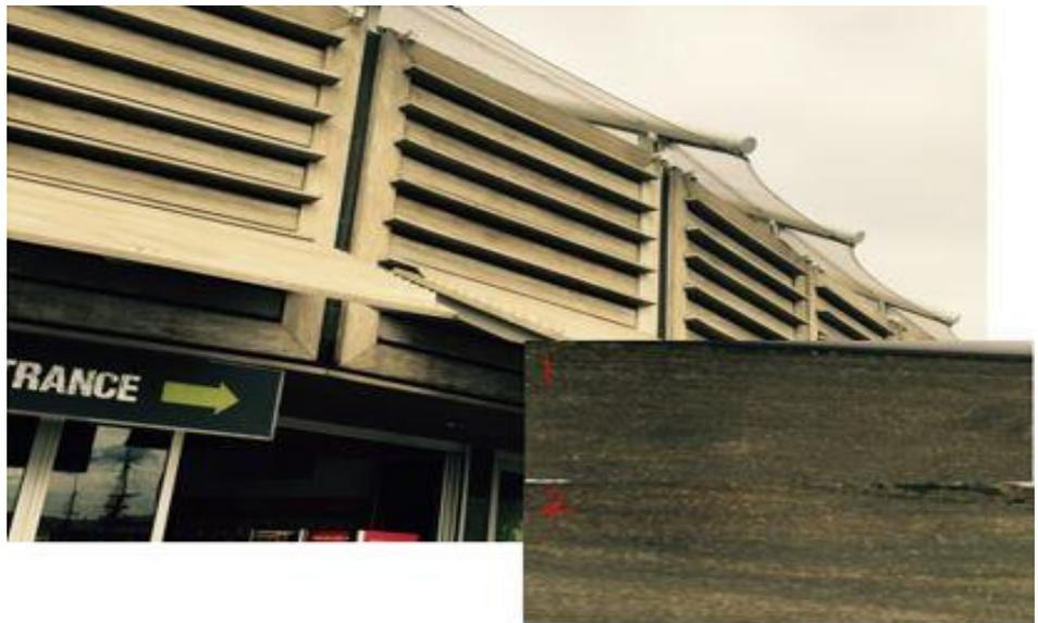
**Sample 1** - The Image of the surface after 10 years of exposure facing North/West (image taken 26 September 2016)
